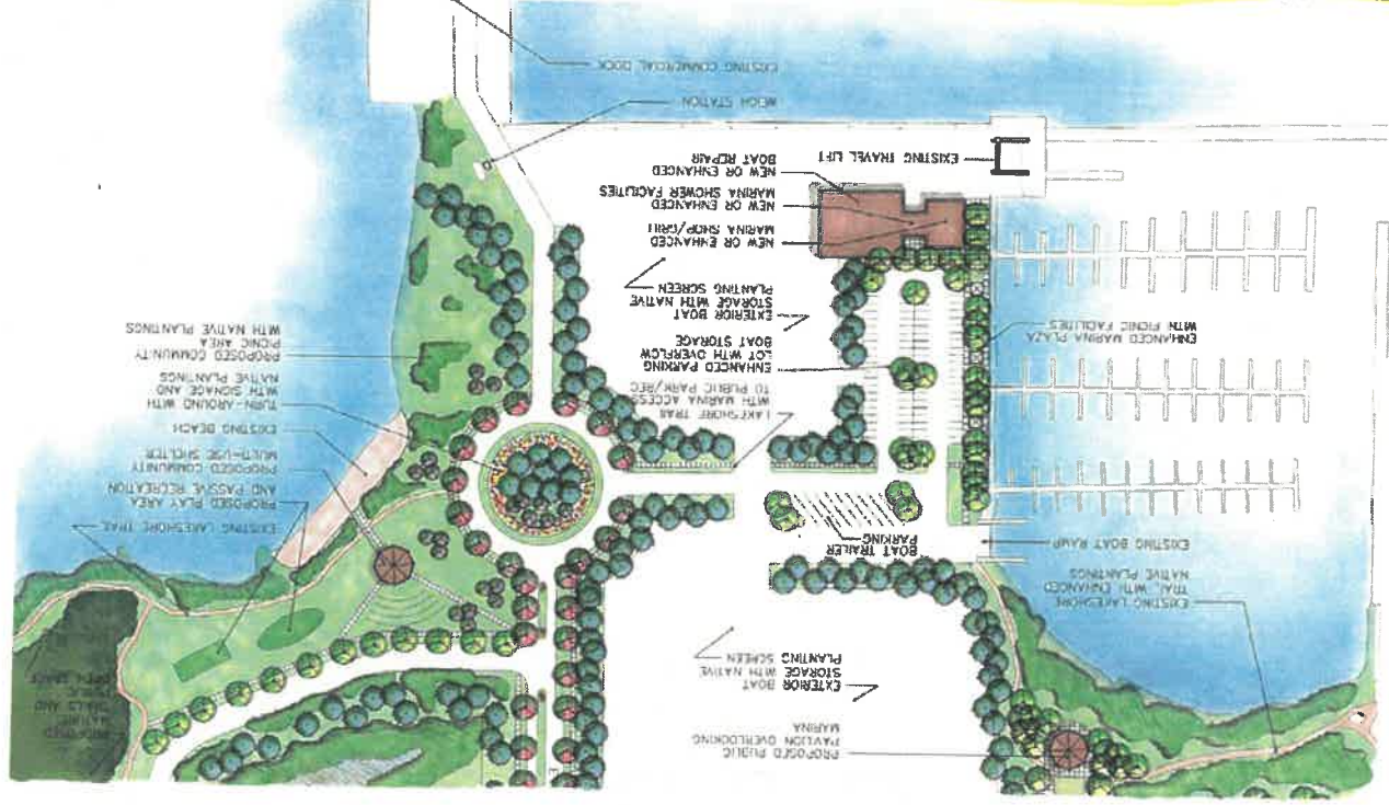
Figure 4-9: Conceptual Sketch Showing Preliminary Ideas for Enhancement of the Marina and Commercial Dock Area
